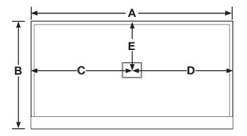
\* Make sure the drain hole in the subfloor or slab is large enough (6" diameter recommended) and aligns with the hole in the shower floor.
